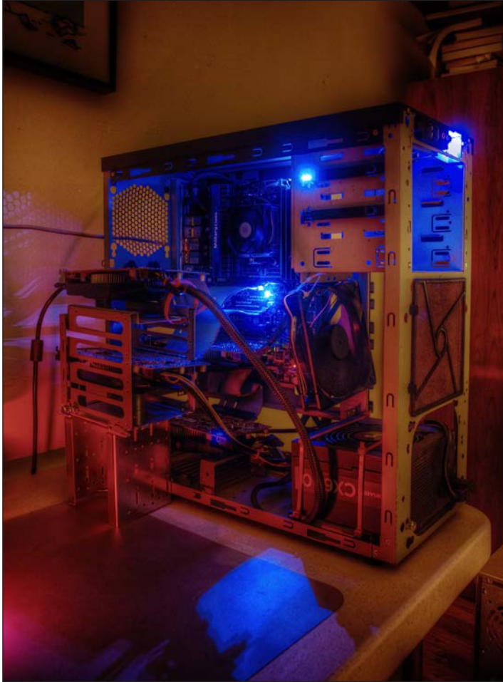
FIG. 3 A “wildcat” home Bitcoin mining rig, from VMAX137’s flickr page. The miner notes that by 2013, “With ASIC and FPGA-based systems coming on line affecting the hash difficulty this miner is no longer effective and has retired from mining.” (Source: [Wildcat home mine] CC Attribution-Noncommercial-NoDerivs 2.0 License. VMAX 137. https://flic.kr/p/nJGgNb .)
